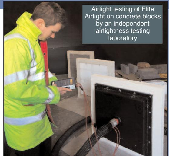
Airtight testing of Elite Airtight on concrete blocks by an independent airtightness testing laboratory
